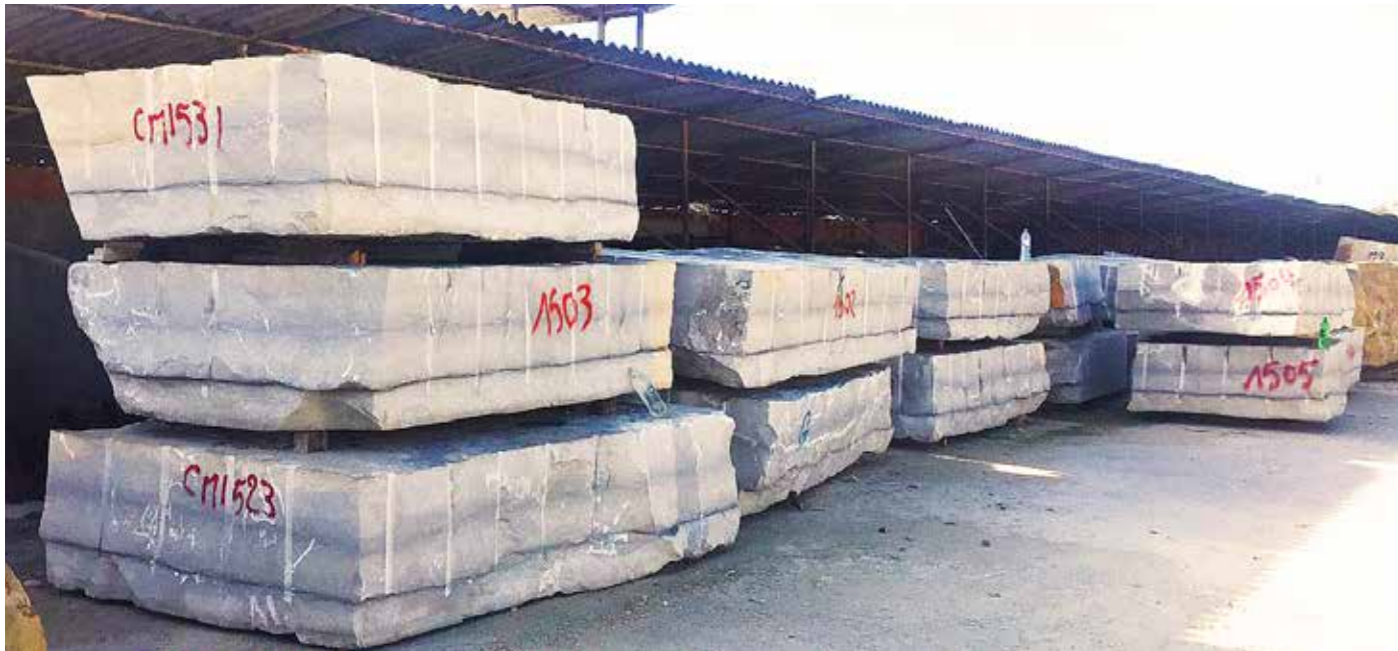
Dorsaf gris blocks - L = max. 3000 - min. 2200 mm / W = 1100 max. - min 300 mm / H = 2000 max. - min 1400 mm
