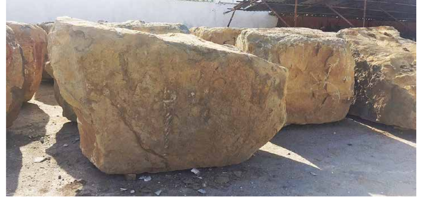
Foussana blocks - L = max. 3000 - min. 1500 mm / W = 1500 max. - min 1000 mm / H = 1600 max. - min 800 mm
